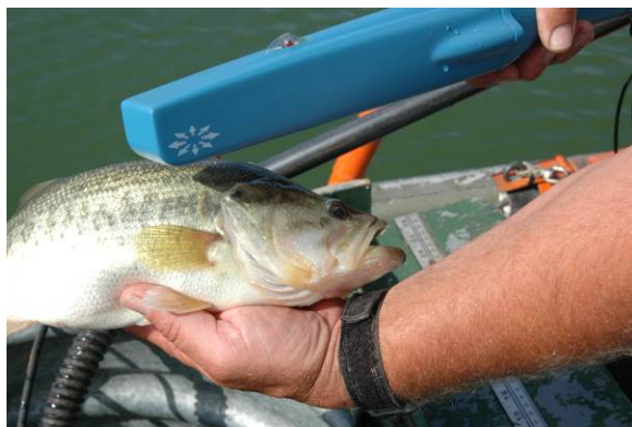
Hidden microwire tags embedded in a fish's cheek often identify it as being from an FWC hatchery, this wand detects the tag.
